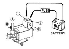
Air passage continuity between **A** and **B** Air passage continuity between A and C Condition 12V direct current supply between terminals 1 and 2 No No No supply
