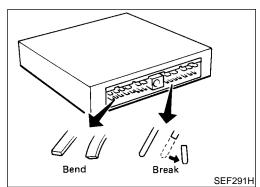
When connecting or disconnecting pin connectors into or from ECM, take care not to damage pin terminals (bend or break).
