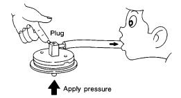
3. If a leakage is noted, replace the valve.
