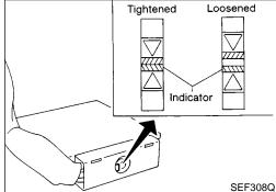
When connecting ECM harness connector, tighten securing bolt until the gap between orange indicators disappears.
