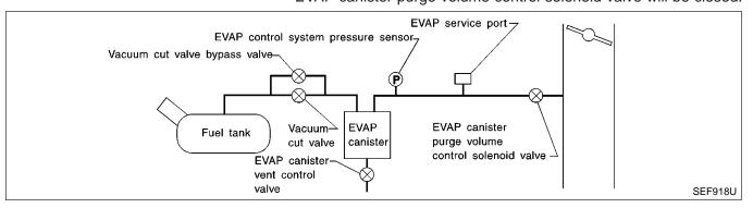
Malfunction is detected when EVAP control system has a leak, EVAP control system does not operate properly.
