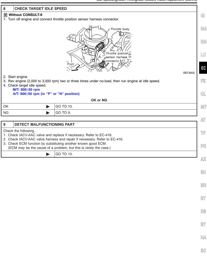
Idle Speed/Ignition Timing/Idle Mixture Ratio Adjustment (Cont'd)
