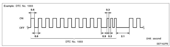
Long (0.6 second) blinking indicates the two LH digits of number and short (0.3 second) blinking indicates the two RH digits of number. For example, the malfunction indicator lamp blinks 10 times for 6 seconds (0.6 sec x 10 times) and then it blinks three times for about 1 second (0.3 sec x 3 times). This indicates the DTC "1003" and refers to the malfunction of the park/neutral position (PNP) switch.
