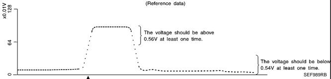
"RR O2 SEN-B1 (-B2)" should be above 0.56V at least once when the "FUEL INJECTION" is +25%. "RR O2 SEN-B1 (-B2)" should be below 0.54V at least once when the "FUEL INJECTION" is -25%.
