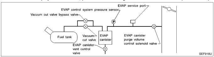
In this evaporative emission (EVAP) control system, purge flow occurs during non-closed throttle conditions. Purge volume is related to air intake volume. Under normal purge conditions (non-closed throttle), the EVAP canister purge volume control solenoid valve is open. Purge flow exposes the EVAP control system pressure sensor to intake manifold vacuum.
