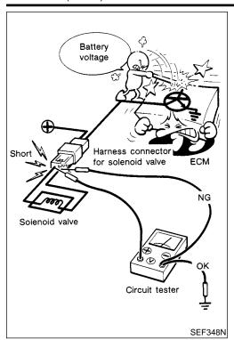
When measuring ECM signals with a circuit tester, never allow the two tester probes to contact.
