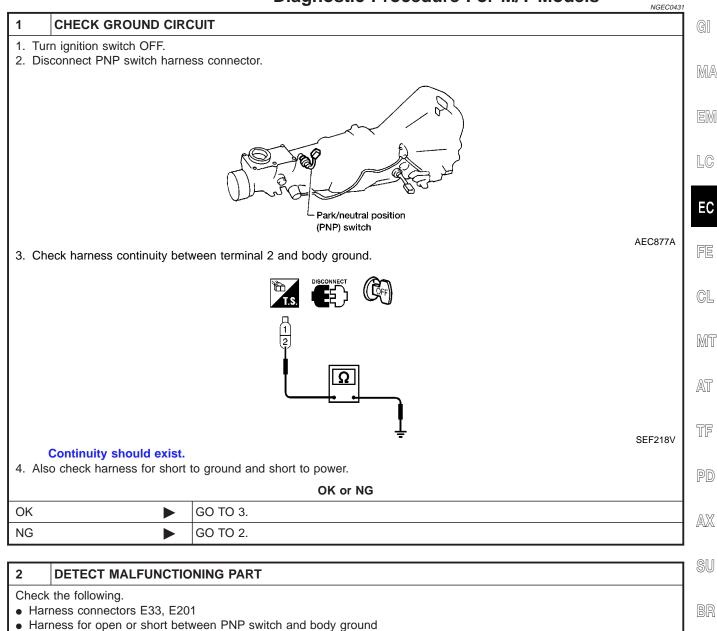
Repair open circuit or short to ground or short to power in harness or connectors.
