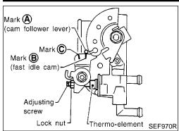
If NG, adjust by turning adjusting screw.
