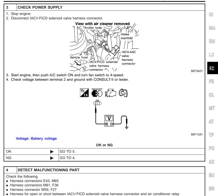
Repair open circuit, short to ground or short to power in harness or connectors.
