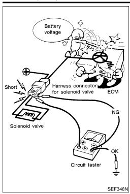
When measuring ECM signals with a circuit tester, never allow the two tester probes to contact.
