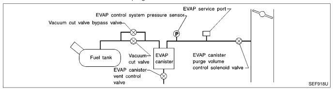
Malfunction is detected when EVAP control system has a very large leak, such as fuel filler cap fell off, EVAP control system does not operate properly.
