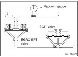
12) Check vacuum gauge while keeping engine speed 2,000 to 2,800 rpm.
