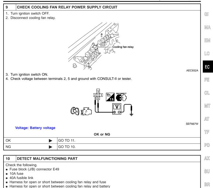
Repair open circuit or short to ground or short to power in harness or connectors.
