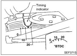
8. Check ignition timing. Refer to "Basic Inspection", EC-669. Make sure that ignition timing is  $15^{\circ} \pm 2^{\circ}$  at  $700 \pm 50$  rpm. If NG, adjust ignition timing and then recheck.
