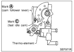
Idle Speed/Ignition Timing/Idle Mixture Ratio Adjustment
