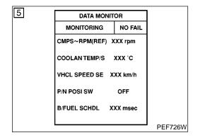
Select "P/N POSI SW" in "DATA MONITOR" mode with CON-SULT-II. Then check the "P/N POSI SW" signal under the following conditions.
