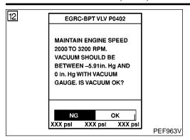
12) Check vacuum gauge while keeping engine speed at 2,400 to 3.200 rpm.
