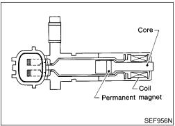
Crankshaft position sensor (OBD)
