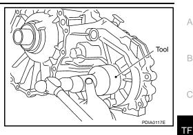
39. Align the matching mark on the front drive shaft with the mark on the companion flange, then install the companion flange.
