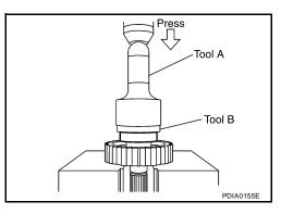
2. Install the front bearing, using Tools.
