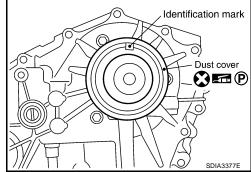
3. Install the new dust cover to the rear case, using Tool.
