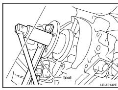
4. Put a matching mark on top of the front drive shaft in line with the mark on the companion flange.
