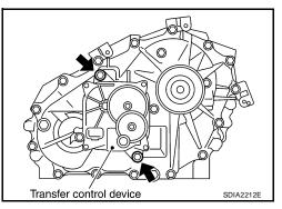
43. Install the drain plug and filler plug with new gaskets to the rear case. Tighten to the specified torque. Refer to <u>TF-112</u>, "COMPONENTS".
