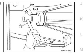
2. Apply petroleum jelly to the circumference of the new dust cover. Position the dust cover using the identification mark as shown.
