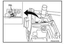
2. Install the baffle plate to the front case. Tighten the bolt to the specified torque. Refer to TF-112, "COMPONENTS" . **CAUTION:**
