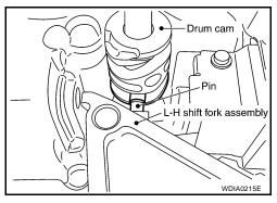
12. Install the L-H shift rod assembly through the L-H shift fork assembly opening to the front case.
