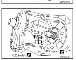
37. Apply sealant to the threads of the 4LO switch (gray with green paint) and ATP switch (black). Then install them to the front case and tighten to the specified torque. Refer to TF-112, "COMPO-<u>NENTS"</u>.
