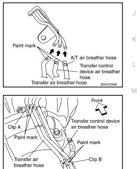
• Install transfer control device air breather hose and transfer air breather hose on clip A and clip B with the paint mark facing upward.
