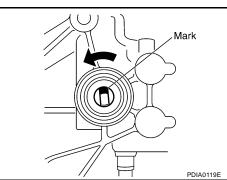
b. Align the transfer control device shaft cutout with the mark on the control shift rod, and install.
