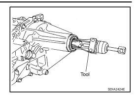
13. Remove the input oil seal from the front case, using suitable tool.
