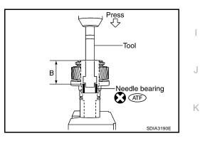
3. Install the carrier bearing to the sun gear, using Tools.
