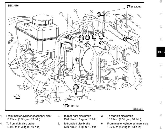
7. ABS actuator and electric unit (control unit)
