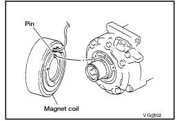
Install the magnet coil harness clip using a screwdriver.
