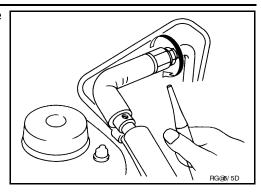
3. Move the probe along each component at a speed of approximately 25 - 50 mm (1 - 2 in)/second as shown.
