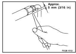
When checking for leaks, circle each fitting completely with the probe as shown.
