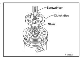
5. Install the clutch pulley bolt using Tool, to prevent the clutch disc from turning and tighten the bolt to specification. Refer to <a href="HA-29">HA-29</a>. "Component".
