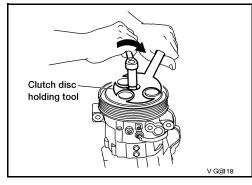
6. Check the pulley clearance all the way around the clutch disc as shown.
