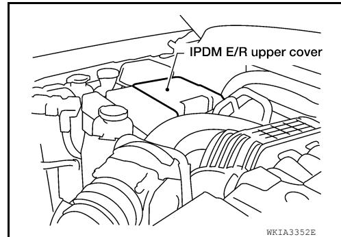
3. Release 2 clips and pull IPDM E/R up from case.
