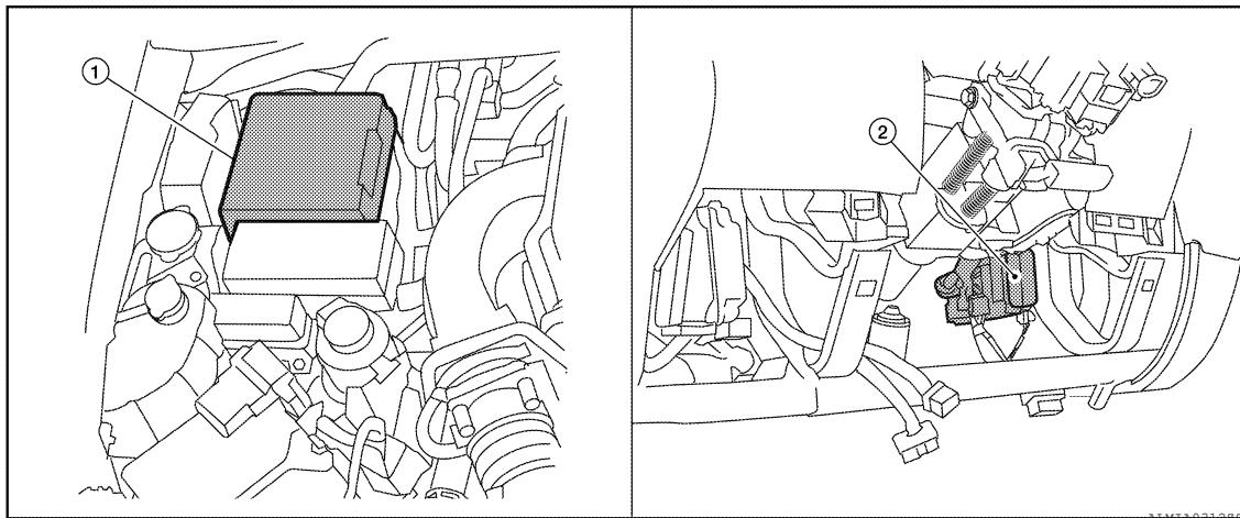
1. IPDM E/R (contains ignition relay) E118, E119, E120, E121, E122, E123, E124
